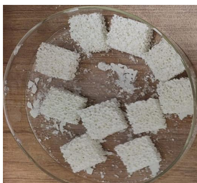
Figure 1. Sintering of the graft at 1200 °C for 3 hours
